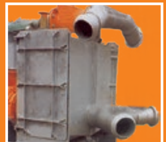
Air Separation Chamber
